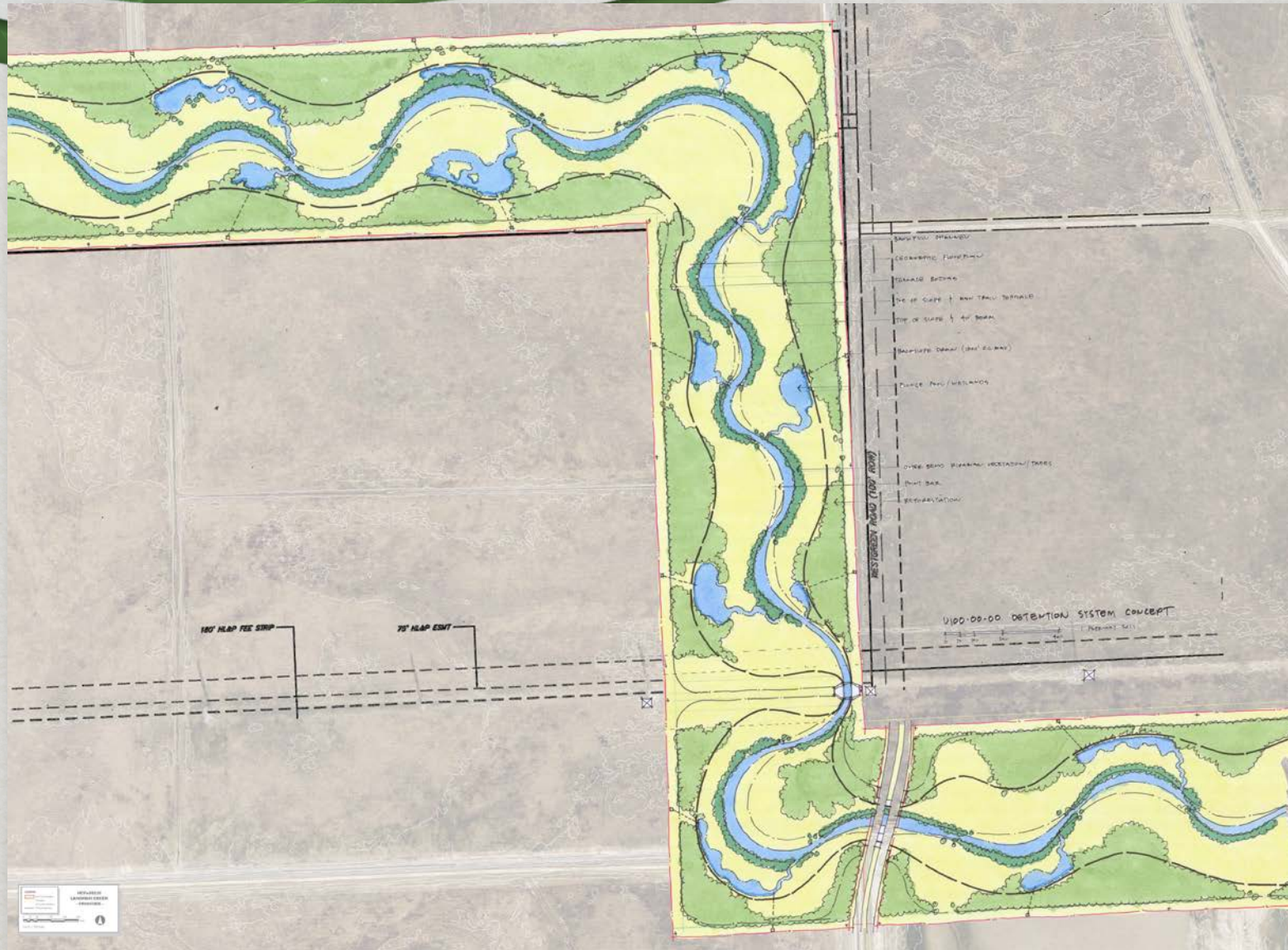
Meandering Stream within Straight Flood Control Channel
