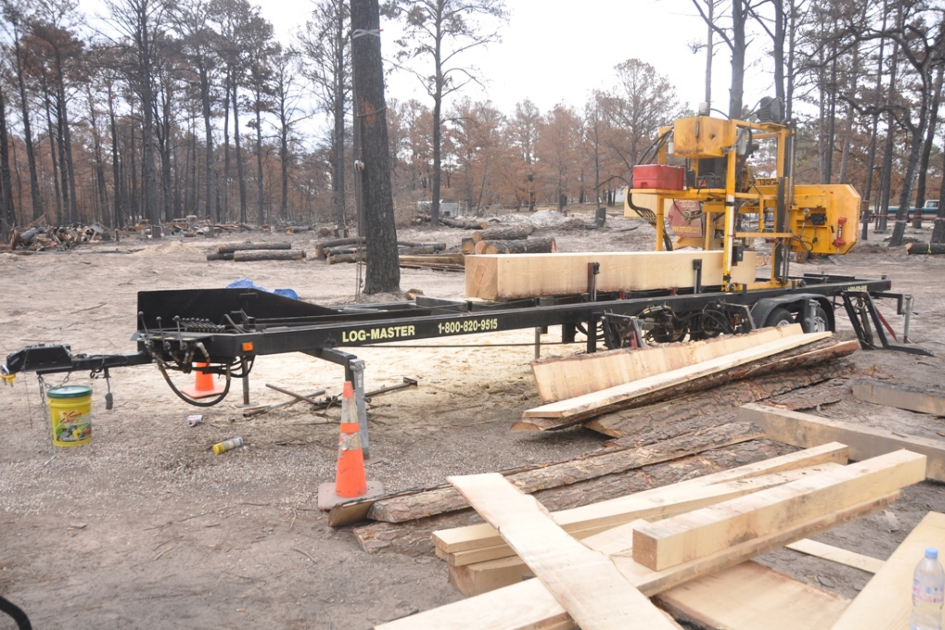
This portable sawmill was used to utilize some of the dead trees.
